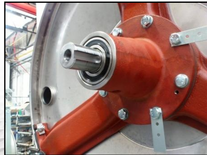
Shaft with groove (RX180-280 /100G)
